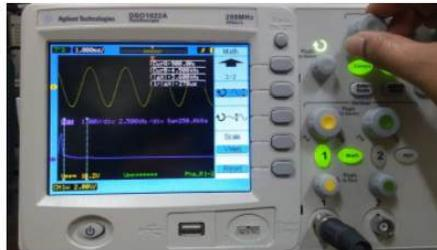
Viewing Fast Fourier Transform on the DSO
