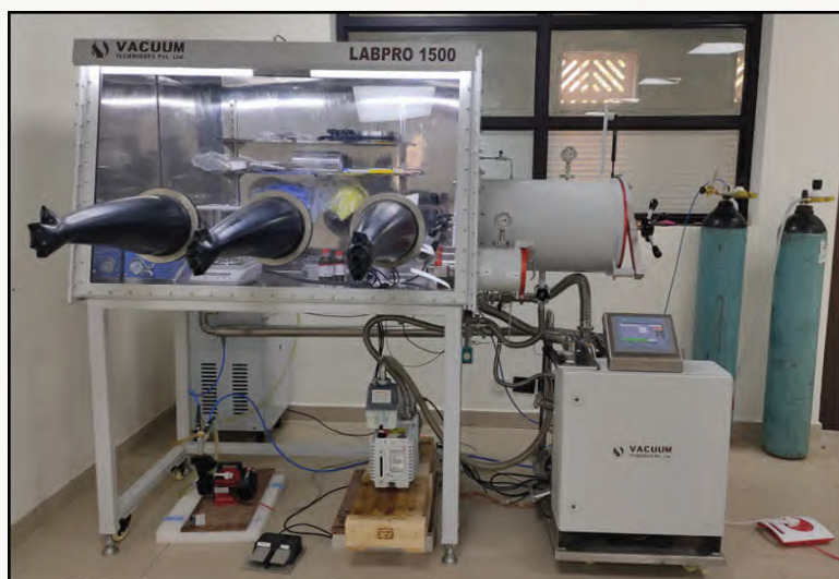
Three-port Glove Box system for the fabrication of Li-ion batteries
