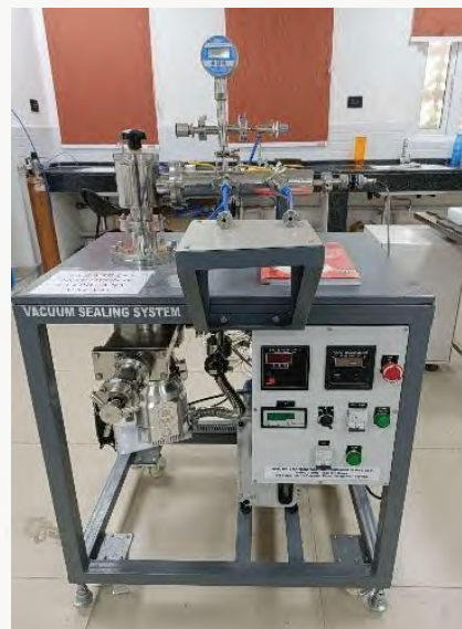
Vacuum Sealing System for Quartz/Glass Pinching (Four Tubes at a time)
