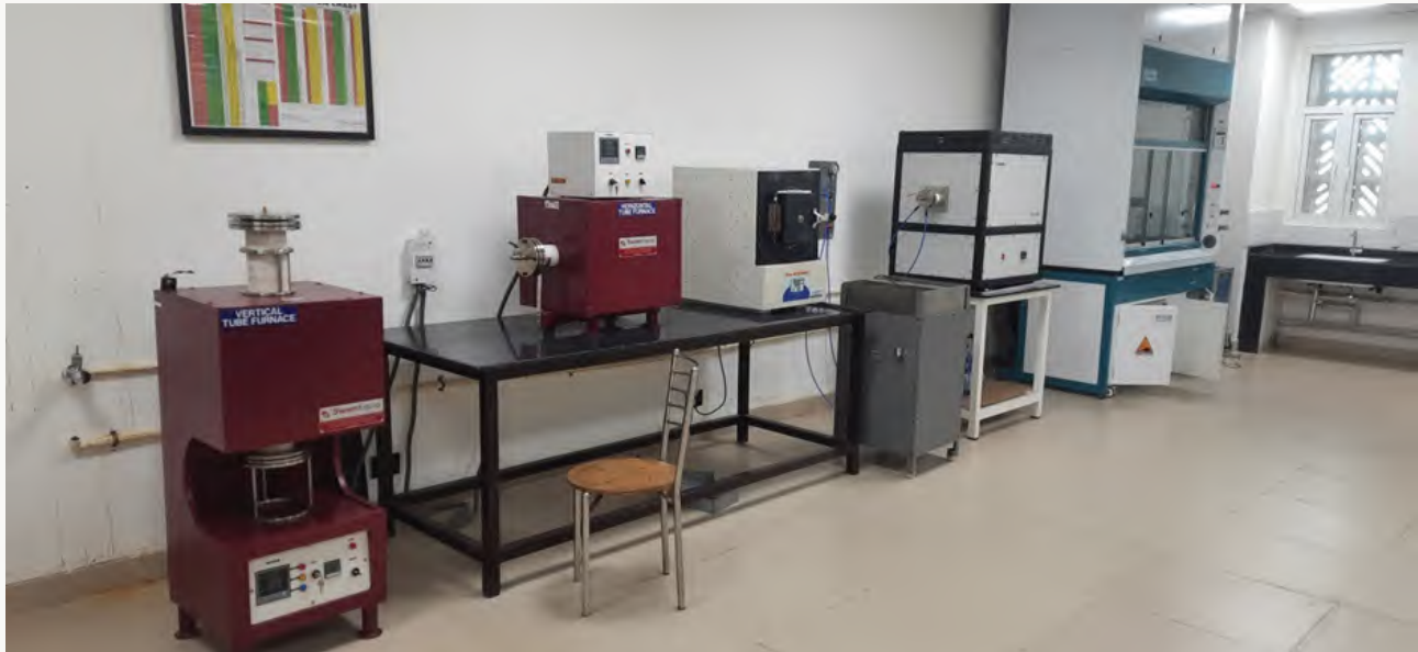
Heat treatment lab showing fume hood, muffle and tubular furnaces
