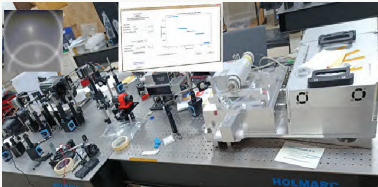
(a) Entangled photons generation using Femtosecond Laser along with single photon detectors (Insert: SPDC ring and GUI for Time-stamping)
