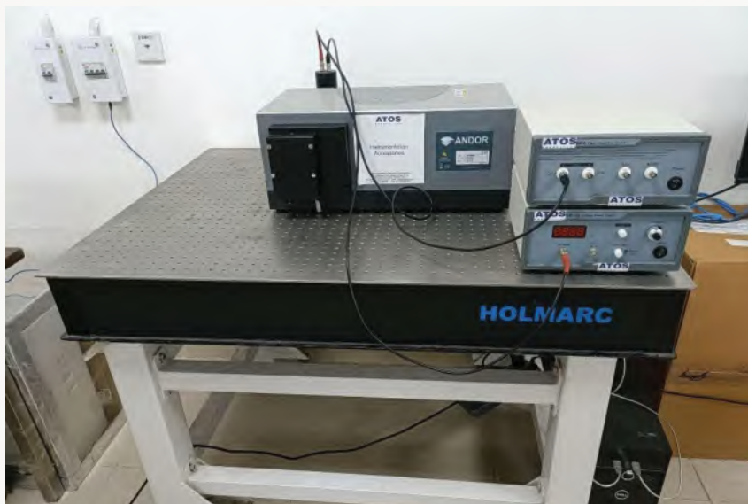
High Resolution UV-Visible Monochromator (Focal Length 500 mm, Aperture Ratio f/6.5, Wavelength coverage 190 nm- 900 nm, Spectral Resolution 0.05 nm with 10 mm wide slits)
