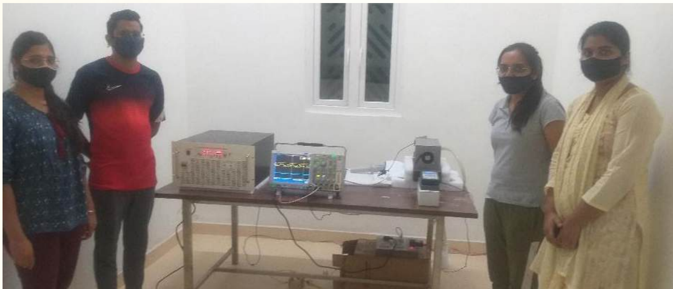
Fig. Electrical Characterization set-up for the testing of DBD systems
