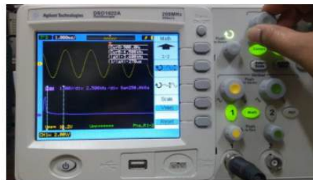
Viewing Fast Fourier Transform on the DSO
