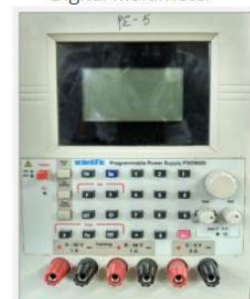
DC Power Supply
