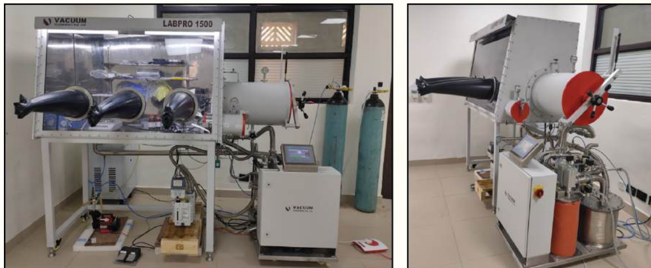
Three-port Glove Box system for the fabrication of Li-ion batteries
