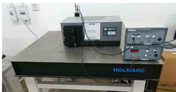
High Resolution UV-Visible Monochromator (Focal Length 500 mm, Aperture Ratio f/6.5 , Wavelength coverage 190 nm- 900 nm, Spectral Resolution 0.05 nm with 10 mm wide slits)
